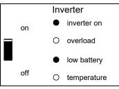
The inverter has switched off due to low battery voltage.
