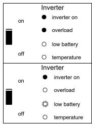
The inverter is switched off due to overload or short circuit.
