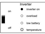
The internal temperature is reaching a critical level.
