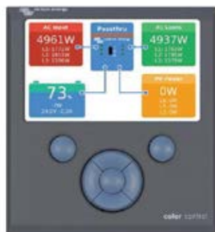
Color Control GX, showing a PV application
